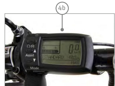
LCD control panel
