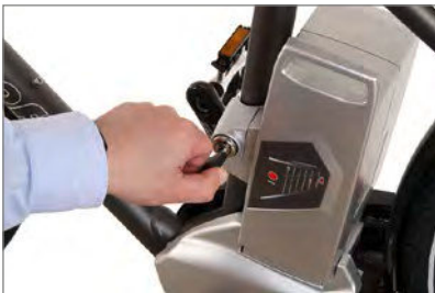
Unlocking the battery
